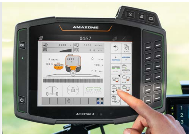
Activering van DirectInject in de terminal AmaTron 4
